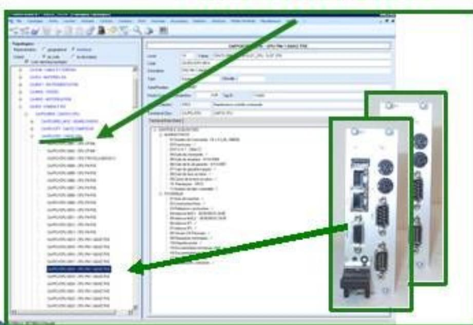
This diagram illustrates the mapping between functional classes and physical hardware. A green arrow points from the 'Functional Class' section above to a list of functional classes on the left, which are then mapped to specific hardware components on the right.
