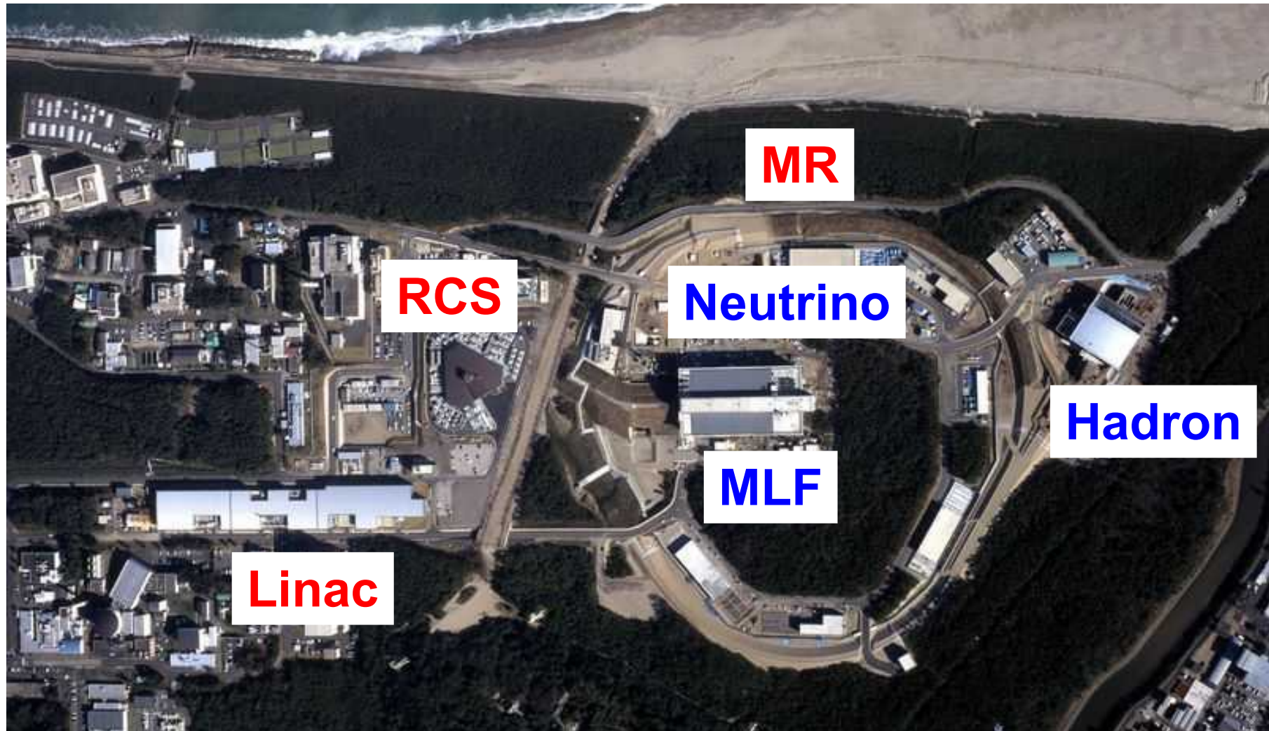
Fig. 1: The beams from the RCS are delivered to the MLF (materials and life science facility) and MR. Typically 4 pulses to MR, 87 pulses to MLF.
