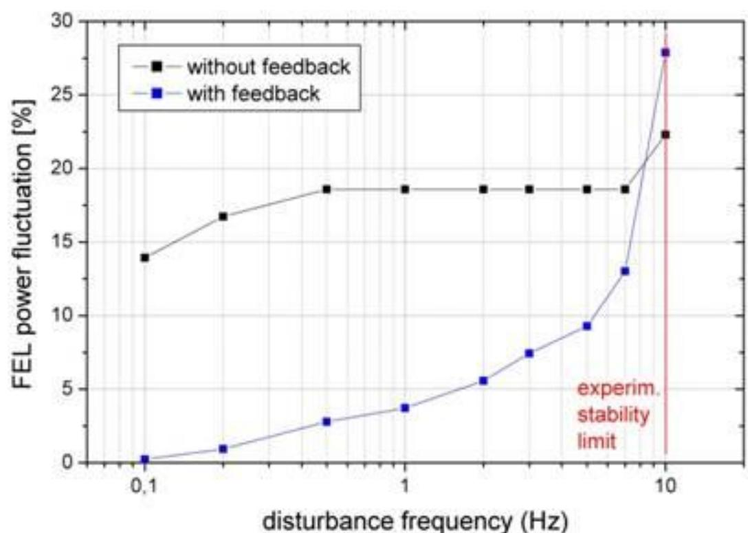
frequency response measured by vertical e-beam modulation
