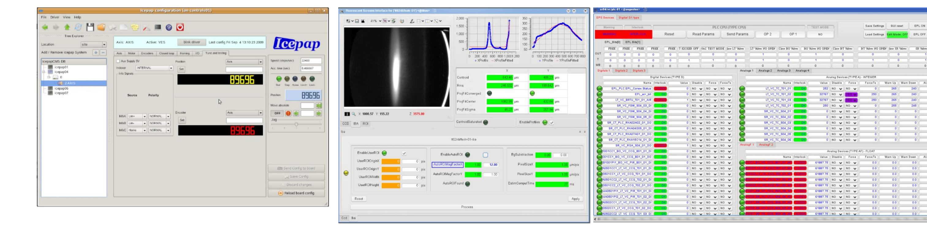
"Stand-Alone" applications. IcepapCMS. *Icepap* is the standard motor controller at Alba. The hardware has been developed at the **ESRF**, and the **configuration** software at Alba (Icepapcms). Many parameters, some of them critical, must be configured before using a motor, like current, encoders, limits, etc. It manages a database with historical configurations; supports motor catalogs and has a tool for online tests. Icepapcms is built with the same standard tools.
