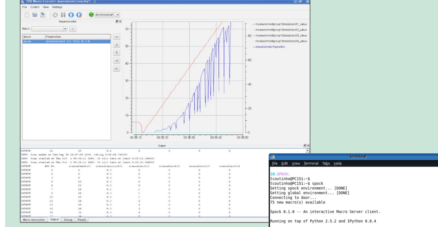
**Spock** is a IPython based **CLI** for **Sardana**. It communicates with the macroserver through one of its doors. Because it is IPython based, all CLI niceties (like word completion on Tab, command history on Up, Down arrows) are automatically available which makes it very easy for spock to mimic SPECs UI. The user executes 'magic' commands (like scans, alignment procedures) in the command line which spock translates to execution of macros inside the macroserver.
