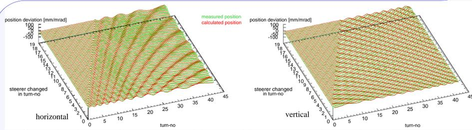
Comparison between the simulation and the actual beam responses due to a change of one steerer kick at a time in the first 19 turns. The right axis denotes the turn number in the HDSM, the upright axis the beam position variations due to a change of one steerer, whose position (in turn-no) is noted at the left axis (there are 4 steerers in each turn). The green lines show the measured beam position deviations, the red ones the deviations calculated by the adapted HDSM simulation.
