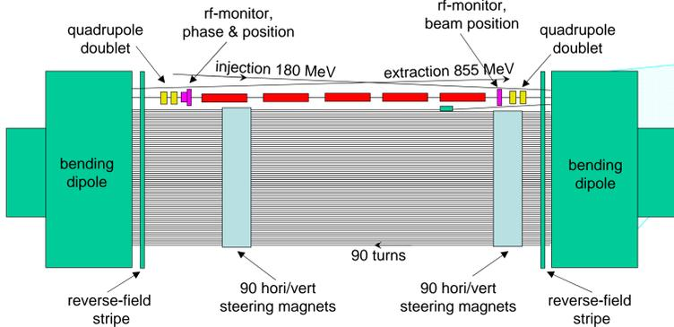
The 3rd RTM stage with an output energy of 855 MeV is in operation since 1990 and serves now as injector for the HDSM.
