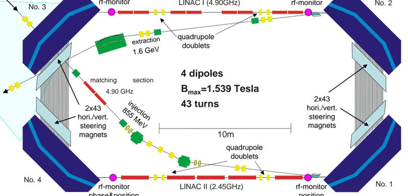
The 4th stage, boosting the energy from 0.855 GeV to 1.6 GeV, was built in parallel to regular operation of the first 3 RTMs. Its commissioning started in Dec 2006 and since Feb 2007 it is in routine operation for nuclear physics experiments.
