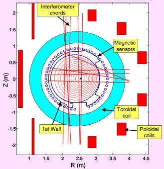
Integration of inductiv Magnetic measurements: 51 pick-up coils: local B<sub>θ</sub> 51 pick-up coils: loca • 6 toroidal flux loops 2 poloidal flux loops
