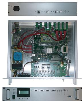
The MX-BPM electronics may be clocked up to 40 kHz to obtain a data rate of 10 kHz in the vertical and the horizontal plane. Its analog bandwidth should allow a correction bandwidth in excess of 100 Hz.
