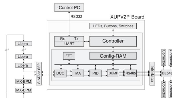
After optimizing the PID controller parameters, we achieved a damping of the 50 Hz line frequency of -20dB. The bandwidth of the correction was limited to approx. 350 Hz. In order to compare BPM capabilities, as the next step we will replace the two Libera BPMs by Bergoz MX-BPMs and XUPV2P boards and repeat the same measurements.
