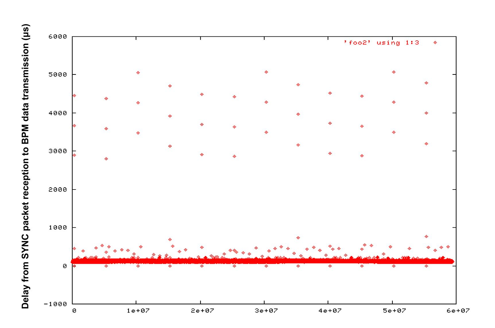
This graph shows network traffic for a single slave of the feedback system operating at 1kHz.
